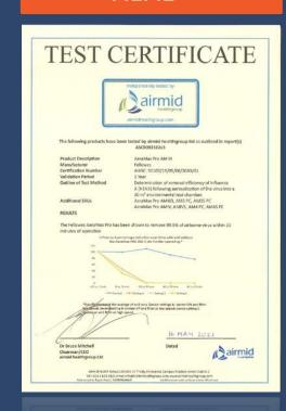
'Fellowes AeraMax Pro air purifiers were demonstrated through independent laboratory testing to be effective in reducing aerosolized airborne concentration of Human Coronavirus 229E in a test chamber, reaching 99.99% airborne reduction within 1 hour of operation.
